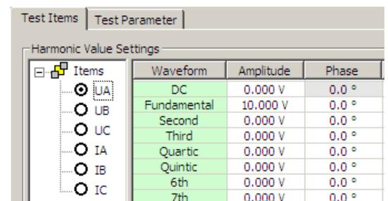
Set amplitude and phase of harmonic in this page. Data phase of the state selected on the left of diagram stands
