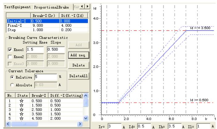
After completing the set of searching range, selecting 'Add Sequence' or "Add" for putting the data of search line in the testing data list. Then selecting 'start the test'. Selecting 'delete' or 'output all' for deleting all single or the whole search lines selected.
