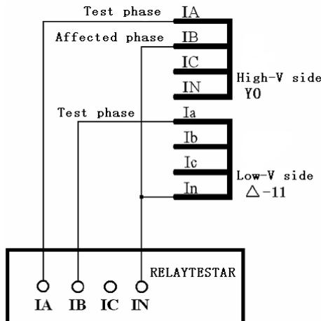
Δ side has phase adjustment, connecting in single phase adjustment, connecting in single phase short circuit mode.
