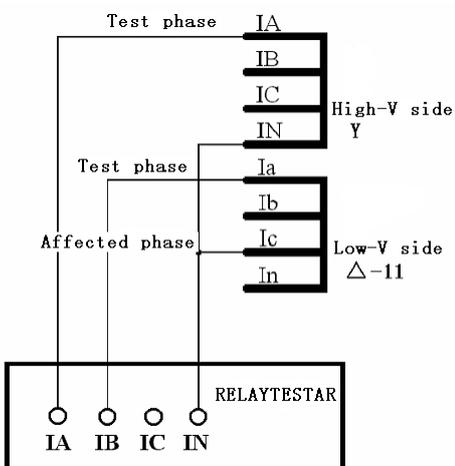
Y side has phase adjustment, not zero sequence connection in single phase circuit mode.
