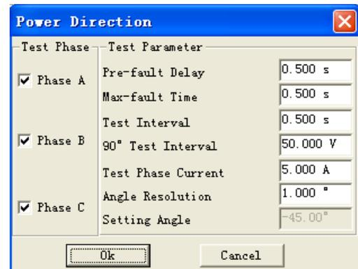
In this item, tests are also done in three-phase successively. You can select single phase or all phases synchronously to be test phases. When testing certain phase, only this phase outputs current, and current of other phases is zero.
