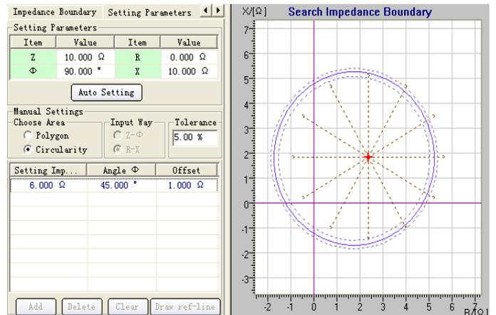
move the cursor to central position of diagram, then click the left key of mouse to set scanning central point as the right diagram shows.
