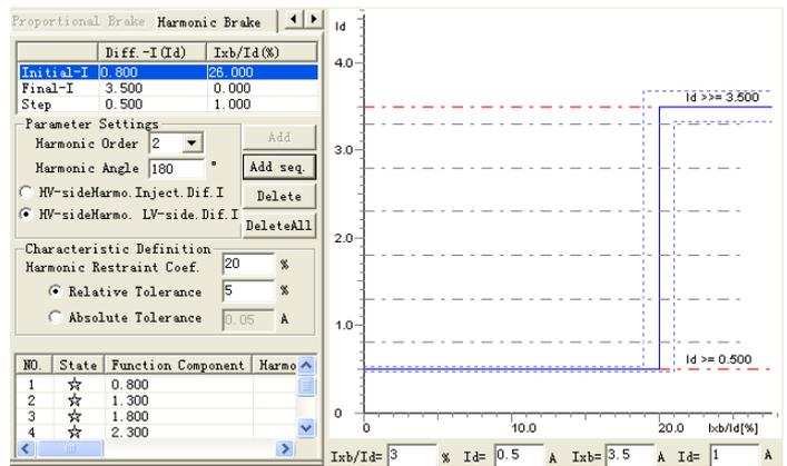
evenly between two horizontal lines, and also every search line should cover action area and non-action area. After completing the set of search range, you should select 'Add Sequence' or 'Add' for filling data of search lines in the testing data list. Selecting 'start the test' for starting the test. Selecting 'delete' or 'output all' for deleting search line.
