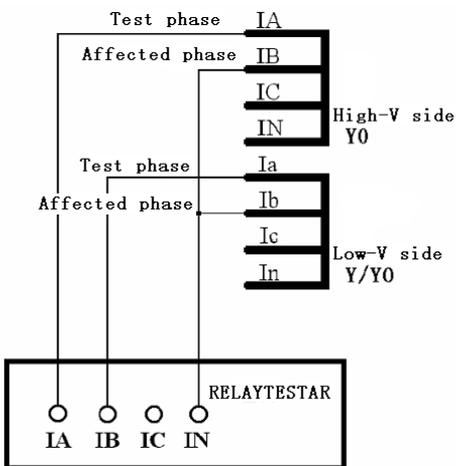
There is phase adjustment on two side, but not zero sequence adjustment
