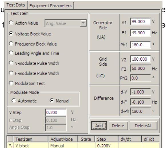
When any one of the above-mentioned parameters needs to be tested, you should always make other two parameters to satisfy synchronization condition in advance. Through changing value of parameters needs to be tested to make the synchronous device to act finally after satisfying fully synchronization requirements.
