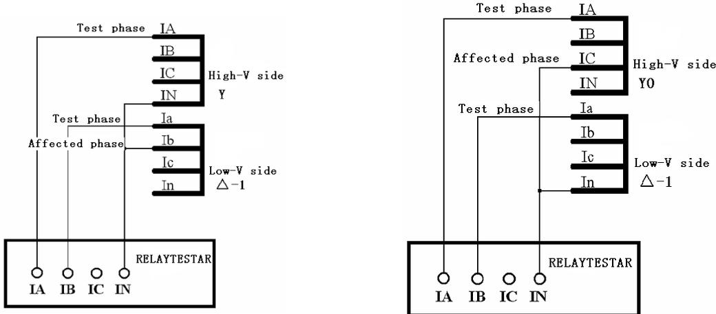
Y side has phase adjustment, not zero sequence. short circuit mode.
