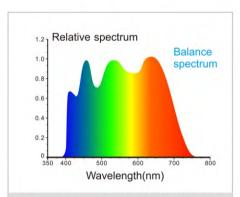
5, Adopt Full spectrum LED light source with blue enhancement The blue-enhanced full-spectrum LED light source ensures sufficient spectral distribution in the visible light range and avoids the lack of spectrum of LEDs in specific wavelength bands.
