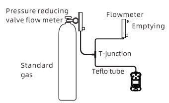
• Press [N/-] to select the gas, then press [Y/+] to enter selected gas calibration screen.
