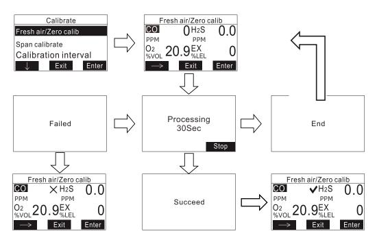
You can terminate the calibration at any time during the countdown by pressing [Y/+] .If the calibration is succeed, it will show av beside the calibrated gas, if the calibration is failed, it will show  $\sqrt{}$  beside the calibrated gas.
