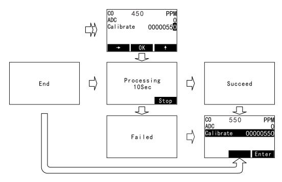
There is a calibrate in the span calibration sub-interface, and the right side is the calibration setting value. The upper part displays the current gas type, real-time concentration value, unit and ADC value.
