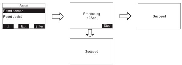
• Press the [Y/+] key to confirm the selection and restore, during which a 10-second countdown will be displayed. During the countdown, press the [Y/+] key again to terminate the restoration setting.
