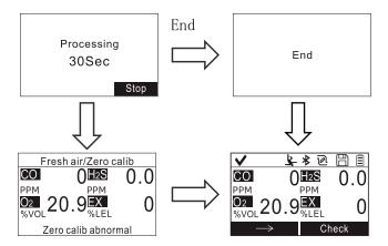
The normal start up of the detector will gradually display the following steps, showing the current settings of the instrument:
