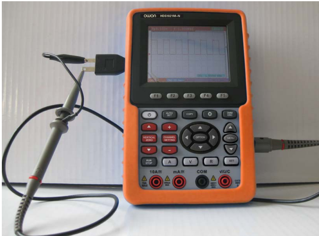
Fig.3. The connection of Square-wave test signal
