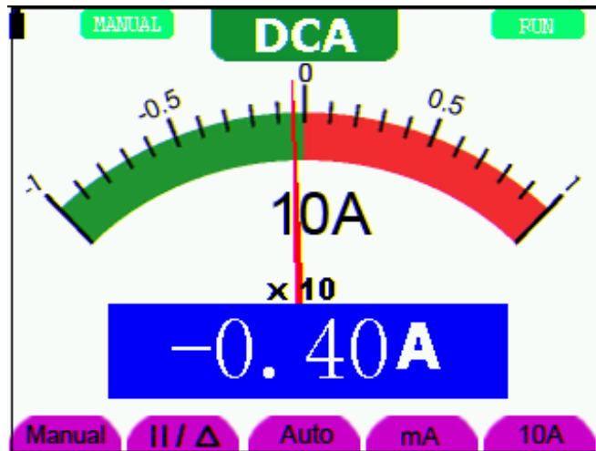
Figure 25: DC Current Measurement for 10A
