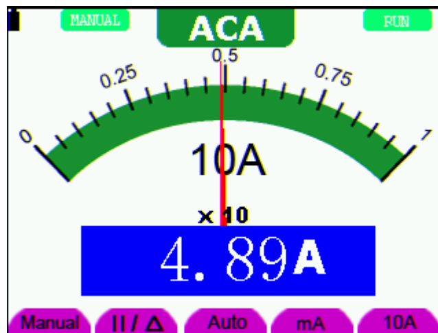
Figure 27: AC Current Measurement for 10A
