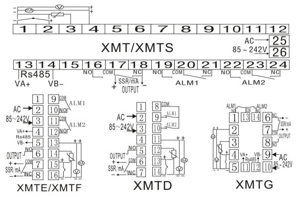
The connection should be subject to the connection diagram attached with the controller.
