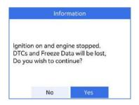
Step two: Select **Yes** and Press OK Button to continue. the device is communicating with the vehicle, and the following prompt interface appears.
