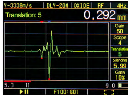
Measurement of oxide scale wall thickness
