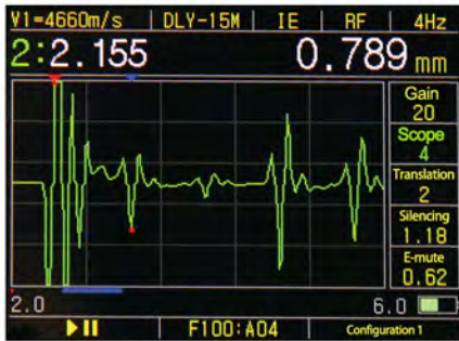
Double-layer thickness measurement of copper-aluminum composite plates
