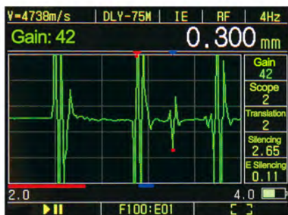
75MHz Probe Measuring Aluminum - Copper Composite Material
