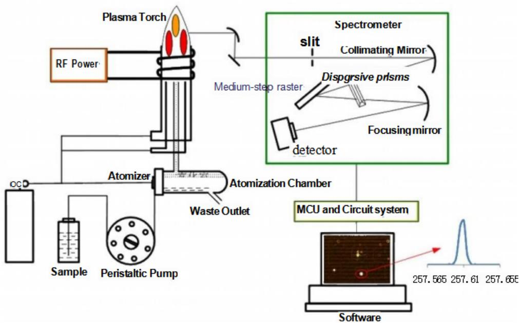
Working principle: the high frequency power generated by the RF generator is added to three layers of
