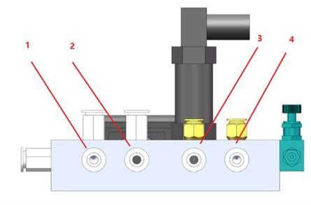
Note: 3 argon gas and 4 purge gas cannot be reversed, otherwise the ignition will fail, and frequent ignition attempts may damage the solid-state power supply.
