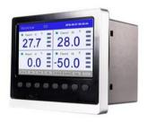
**sisco-PLR- CH48** is a 7 inches TFT true color LCD paperless chart recorder with power supply AC 85~264V (50/60Hz) or DC 12-36V, internal storage 64M bytes flash, 1-48 data channels, 33 kinds of input signals, 18 alarm outputs, 12 analog outputs, RS485/RS232/Ethernet communication output. It has additional functions of File List, Print, Backup, Configuration, etc.
