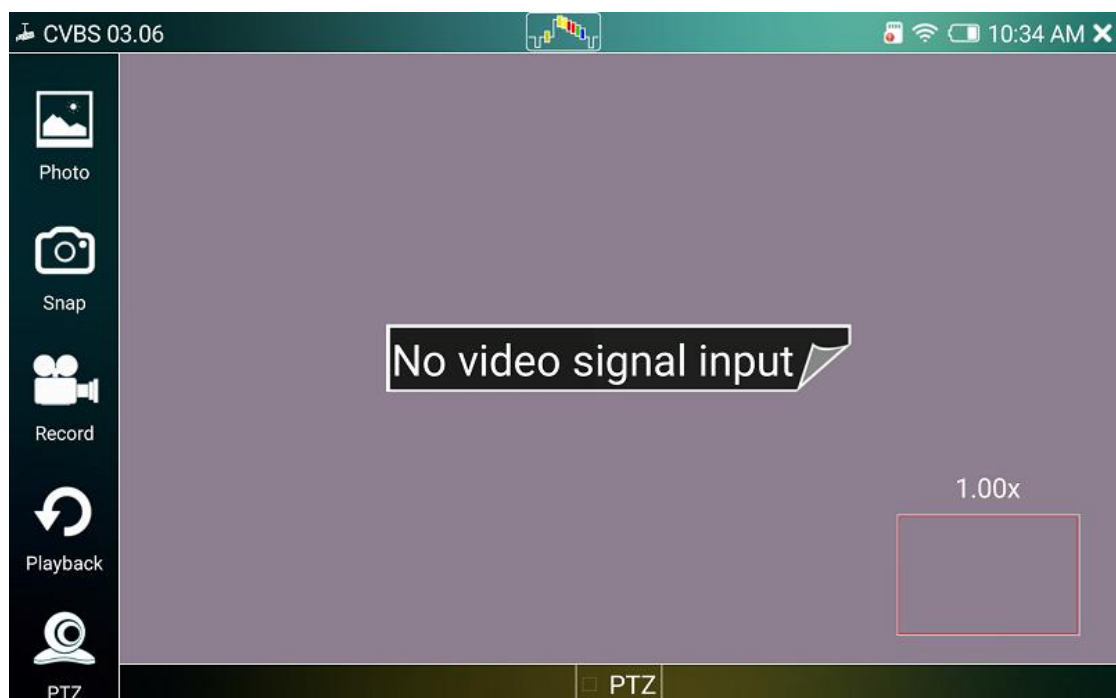
Figure 8 CVBS Analog Video Test Main Interface
