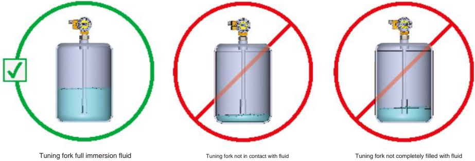
Figure 2-14: Meter placement (immersed in fluid)
