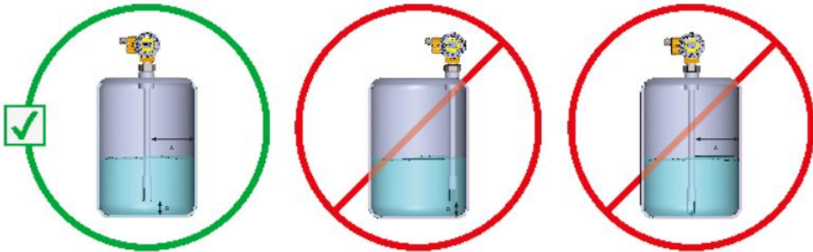
Figure 2-13: Instrument placement (away from tank wall)
