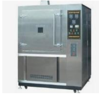
Xenon lamp aging test chamber
