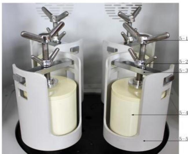
Figure 5. Actual View of the Grinding Jar Holder and Clamping Device of the Vertical Planetary Ball Mill
