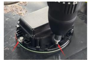
Fixed hexagonal dovetail screw All four screws need to be fixed
