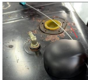
Insert the seal according to the direction of the arrow
