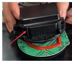
Insert the sensor into the fuel tank and align it with the gasket
